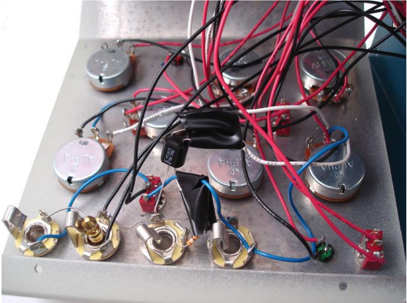
Install the vactrol and 390ohm resistor directly inside the case. Use electrical tape or heat shrink tubing to protect the wires. Make sure the positive side of the vactrol is attached to the positive Jack terminal. See the [connection diagram](#) for more clarification. Finally solder wires to the battery holder, attach the standoffs to the pcb and screw together the case.
