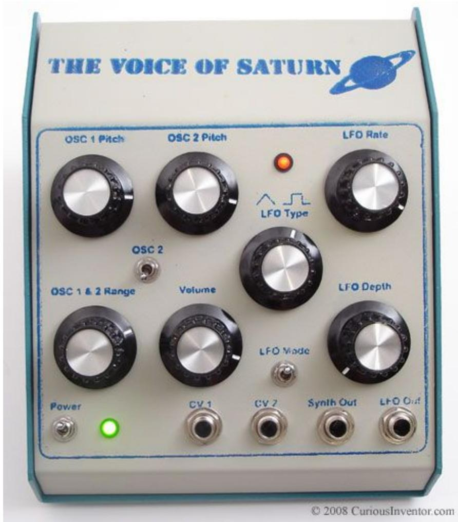
When you first turn it on, the green light should be solid and the red should blink slowly if the LFO Rate is all the way to the left (counter-clockwise). Some knob arrangements don't product any sound at all; set the knobs and switches as shown above to get something.
