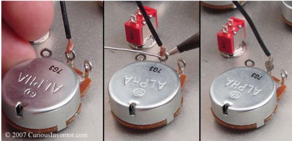
First loop the wire through and bend it to hold it in place, then heat the joint from one side and apply solder to the other. Again, it will help to put a bit of solder between the iron tip and connection to act as a heat bridge.
