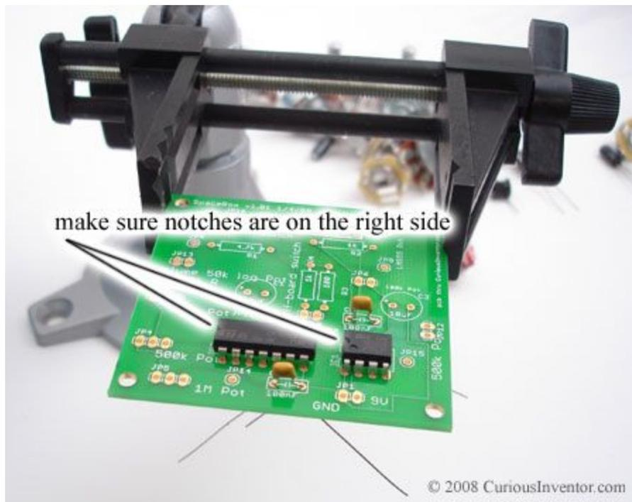
Last, add the ICs making sure to line up the notches on the chips with the markings on the pcb. If available, use IC sockets to further protect the chips from damage.
