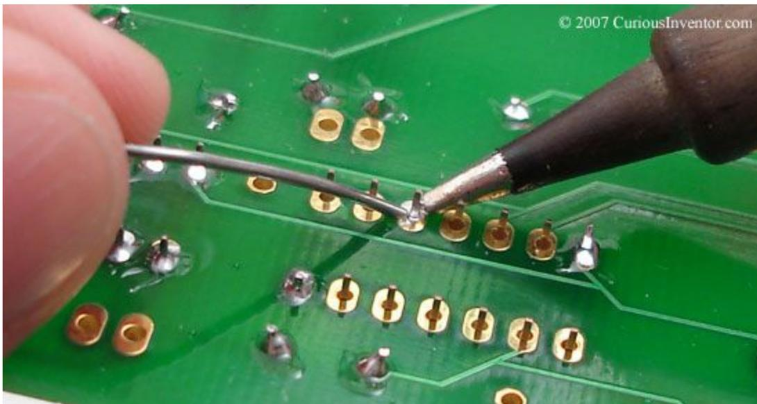
Tin the tip, or in other words, add a bit of solder to the tip, first. This small amount of solder forms a "heat bridge" to help conduct heat from the tip to the pad and component lead. When you first contact the parts with the iron tip, it's helpful to first place some solder in
