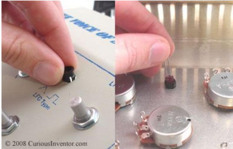
Install the LED holders from the outside, then press the LEDs into them from the inside until they snap in place.
