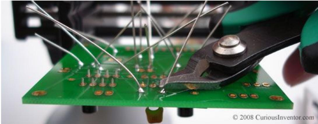
Cut off the leads as you go with flush cutters. Watch out for flying leads; safety glass are actually not over-precious for this, although we generally just hold the lead with fingers to keep it from flying off.
